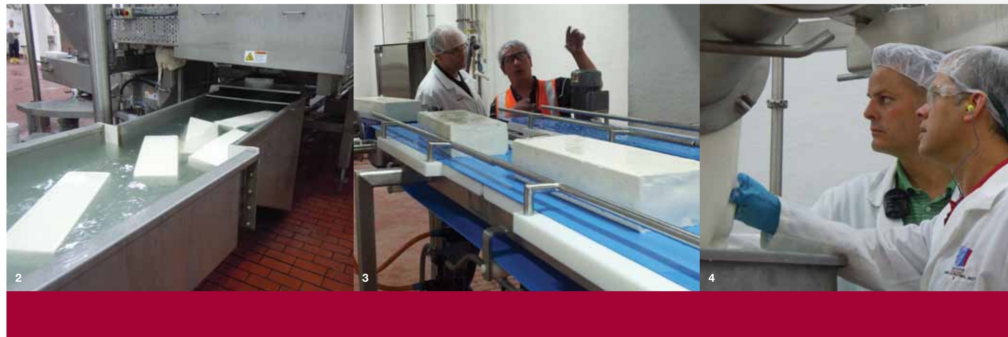
1. Davisco staff on hand to observe the first mozzarella blocks emerge during the cheese molding process. 2. The mozzarella cheese is submerged in a brine solution before entering the cage system where it cools and cures prior to packaging. 3. Marvin Bartlett (director of engineering) and Jared Brandt (project manager). 4. Bill Riebesell (Jerome Cheese plant manager) and Troy Ammann (director of cheese operations).
